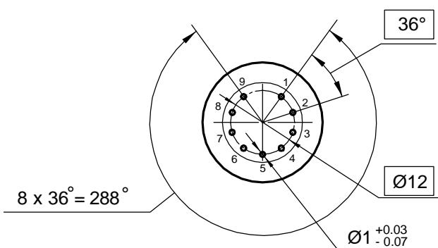
Electrode -to - lead connection diagram
